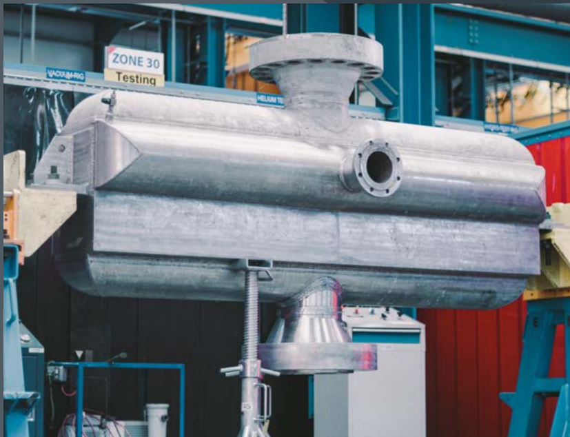
IMAGE: An example of a Meggitt PCHE (Printed Circuit Heat Exchanger).
